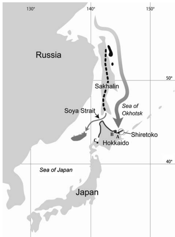
Fig. 1 Schematic presentation of the location of Hokkaido and Sakhalin Islands. The pipeline (broken line) from the Sakhalin oil fields (areas in black) to a port facing Hokkaido and the navigation route of tankers passing through the Soya Strait (thin arrow) are included. The flow of the East Sakhalin Current is shown by the heavy arrow. The Hokkaido coastlines that are at risk of oil contamination from the Sakhalin oil fields are shown by the solid black line. Points A, B, and C indicate the seashores of Shari Town (45°56'N, 144°43'E), Abashiri City (44°02'N, 144°15'E), and Ishikari City (44°55'N, 144°93'E), respectively, where sea sand was sampled
